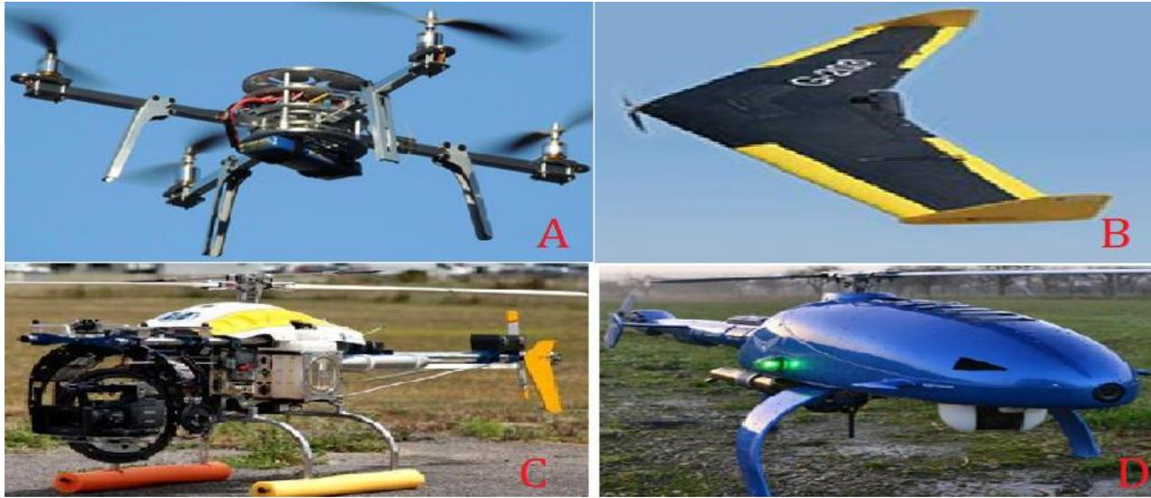
**Figure 1:** Types of drones currently in use: A (Multi Rotor), B (Fixed Wing), C (Single Rotor) and D (Hybrid VTOL). *Source:* CircuitsToday, 2018.
